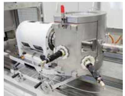
Test cavity with temperature sensors
