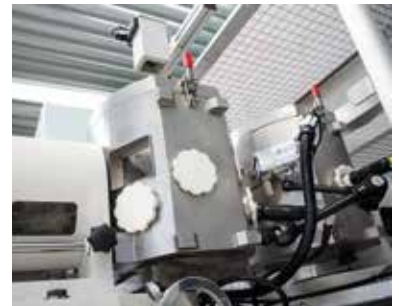
Test cavity with camera system
