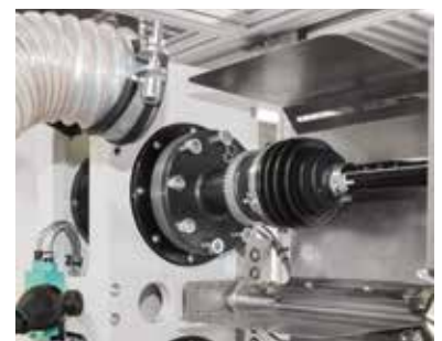
Grease leakage detection and air flow simulation
