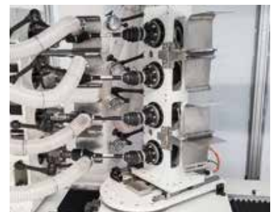
Bearing unit with applied steering angle
