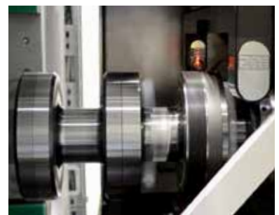
Integrated laser measuring system LC50-DIGILOG for runout measurement
