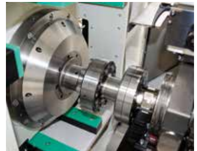
Connecting shaft between load spindle and specimen
