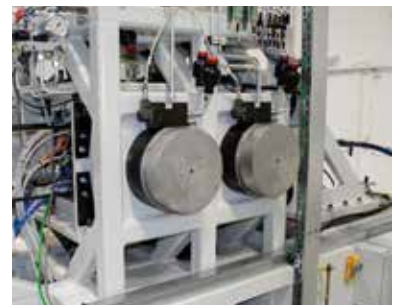
Frame with hydraulic diaphragm cylinders
