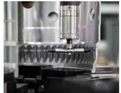
Precise measurements using the compact BLUM touch probe with wear-free measuring mechanism
