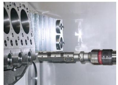
BG61: Solution with up to 8 individual measuring elements
